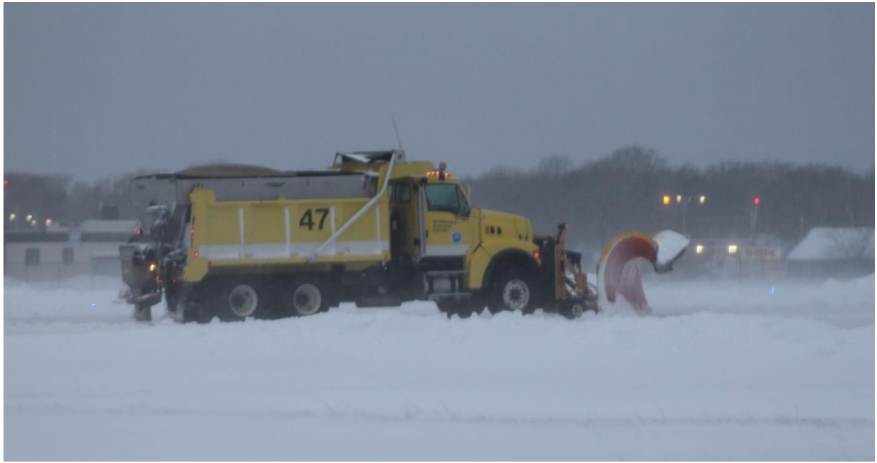
2006 Sterling A Line Diesel Heavy Duty Carrier Vehicle with Plow and Sander
