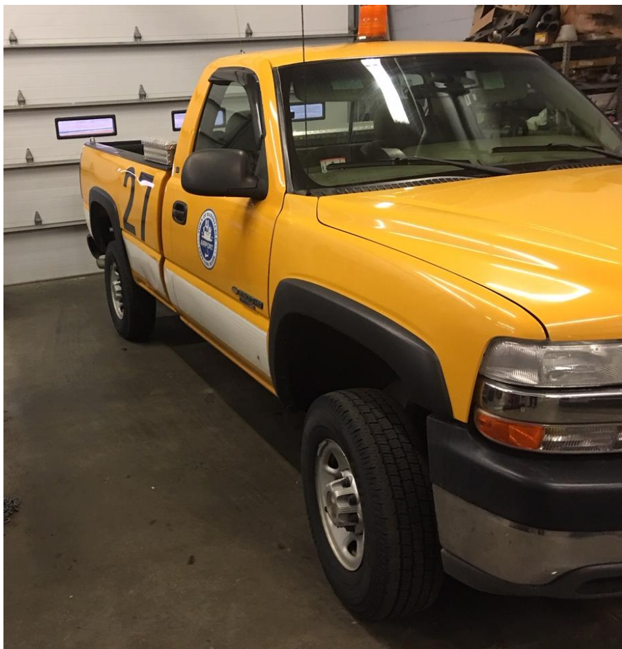
Snow Removal Equipment (SRE) (Chevy 2500HD – Heavy Duty Vehicle with Plow– Airport Vehicle #27 Circa 2001)
