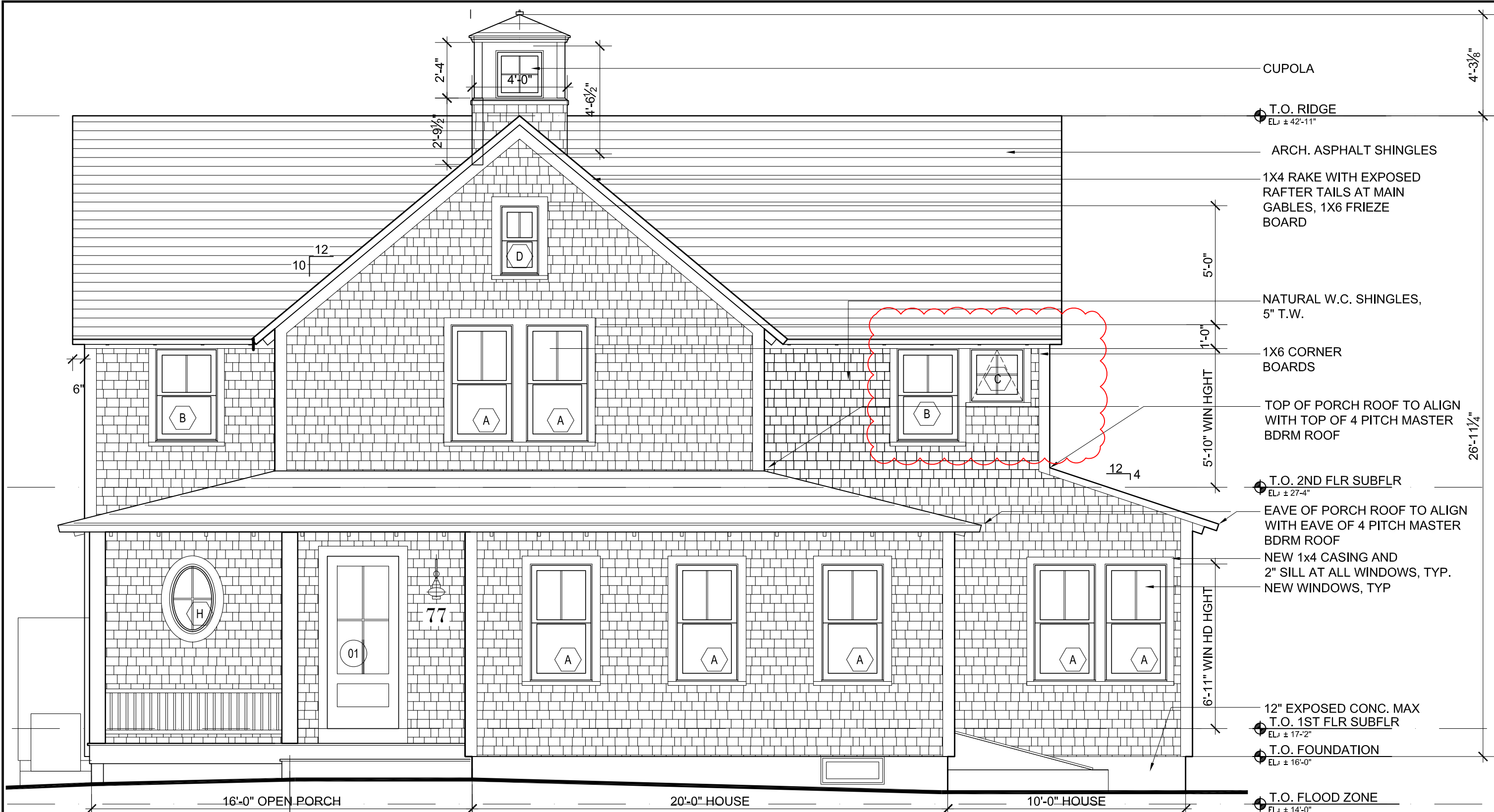
1 SOUTH ELEVATION (SUNSET LN) A2.0 1/4" = 1'-0"
